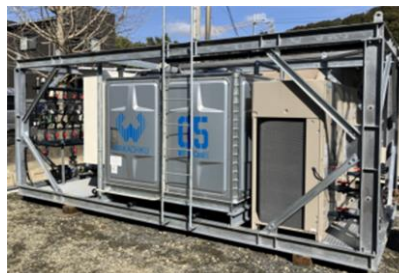
AI water-temperature-controlled pipe-cleaning system
